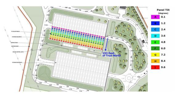
Figure 1: Orientation and tilt of the panel layout used to calculate glint and glare
